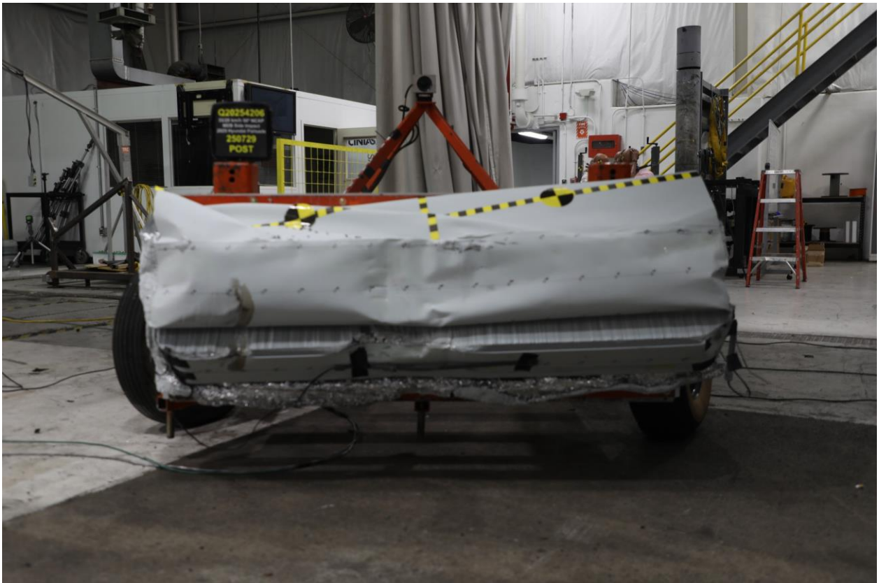
085 Post-Test Front View of MDB Impactor Face
