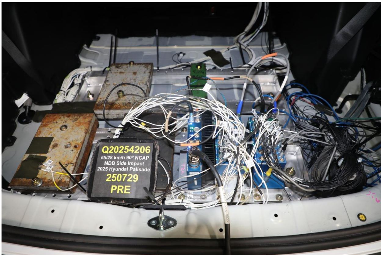
094 Pre-Test Ballast View
